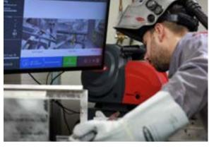
Step-by-step: A display visually shows the work steps in the defined order and the corresponding welding parameters are automatically set.
