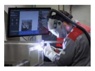
Live monitoring and error alerts enable a quick response and correction if necessary to minimize waste and rework.
